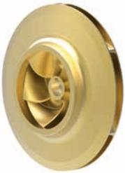
Closed multi-vane impellers made of high-alloyed aluminium bronze (CuAl10Fe5Ni5) are used for clean to slightly contaminated pumped media.
