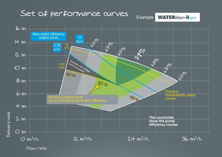
Example for 0.75 kW pump: Previous optimal efficiency level: 58 % New efficiency with full impeller diameter according to shell curve: 68 % => Hydraulic optimisation of the efficiency by 10 % !
